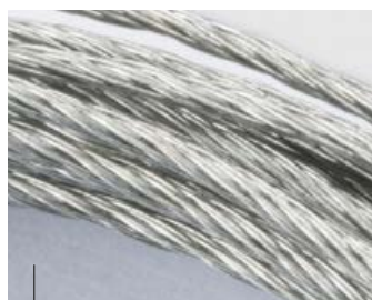
Stahlcord Steel cord
