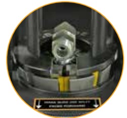
Ideal notched pressure plate when crimping 90 deg. fittings
