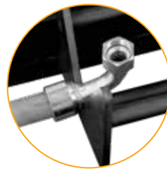
Elbow fitting adapter and the ability to adjust the position of the ram makes it possible to assemble a wide variety of fittings
