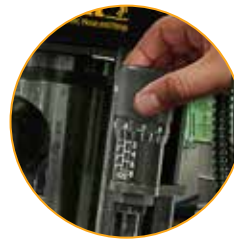
Micrometer is fully adjustable for a precise crimp
