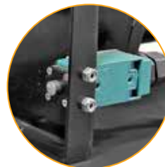
Safety Switch activates and shuts the motor off when the safety shield is opened
