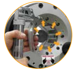
Easy grease maintenance through the 8 lubrication fittings
