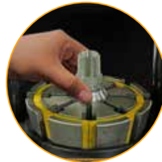
Open design allows the operator to accurately position the fitting prior to crimping
