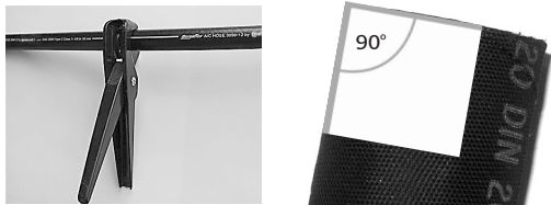
The cut must be made squarely to the hose length.
